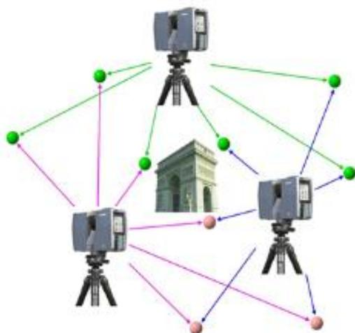
**Figure 4: Connected scanning targets**
