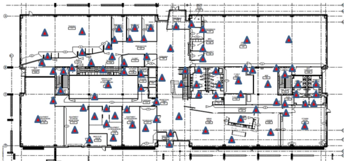
**Figure 3: Scan plan with stations identified**
